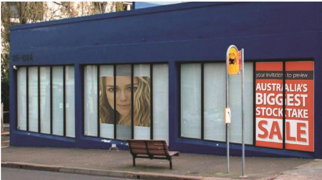
Diagram 6: This picture represents Method 4 approach. The installer in this instance has trimmed the artwork into 3 separate panels, but this time has not trimmed 25mm strips out. This is fine when viewing straight on, but when viewing on an angle as above, a distorted image will appear.
