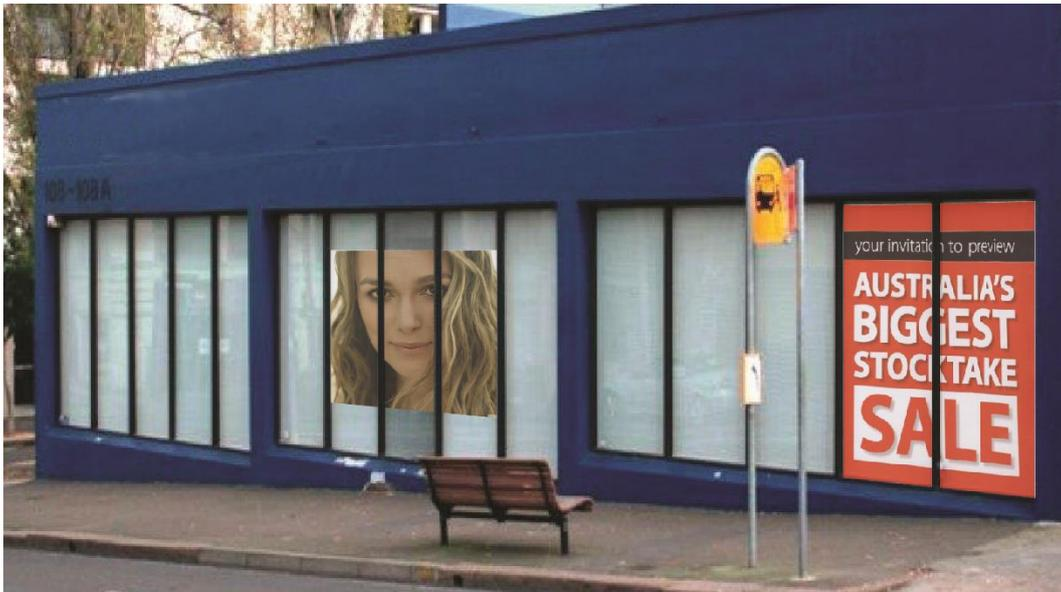
Diagram 5: This picture represents Method 3 approach. Artwork spans the window panes, but installed as three separate panels, with no film on the window frames, rather this has been trimmed out. That is, assuming the window frame is 25mm wide, then the installer has cut out 25mm strips out of the printed graphics, running through the eyes.
