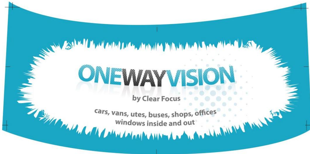
Diagram 2: Recommended artwork layout. Notice the cross hairs, centre marks and bleed. For vehicle windscreens, it is suggested to curve the text to the shape of the windscreen. When installed, the text will appear horizontal. Otherwise, the text will actually curve downwards, looking like a “frown”.
