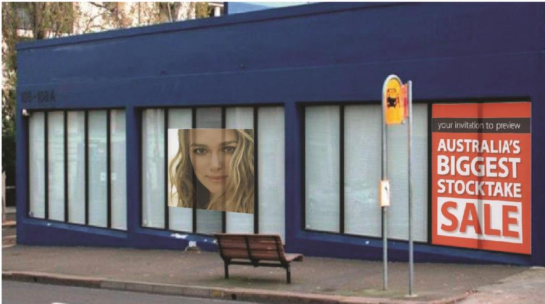
Diagram 3: This picture represents Method 1 approach. Film is applied over the window frames to provide a continuous look to the image. This is recommended when involving faces or features which should not be trimmed out.
