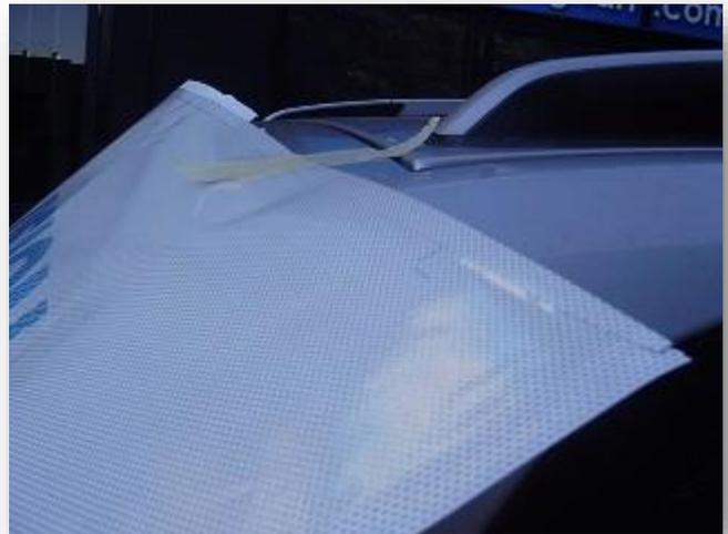
4. OWV film is applied to the exterior side of the windscreen. For rear windscreens, applying over the entire windscreen including mounted brake lights is allowed. Locate the horizontal and vertical centres of the trim area on the OWV film, and on the vehicle windscreen. Mark these centre points with application tape, both on the OWV film and on the vehicle.
