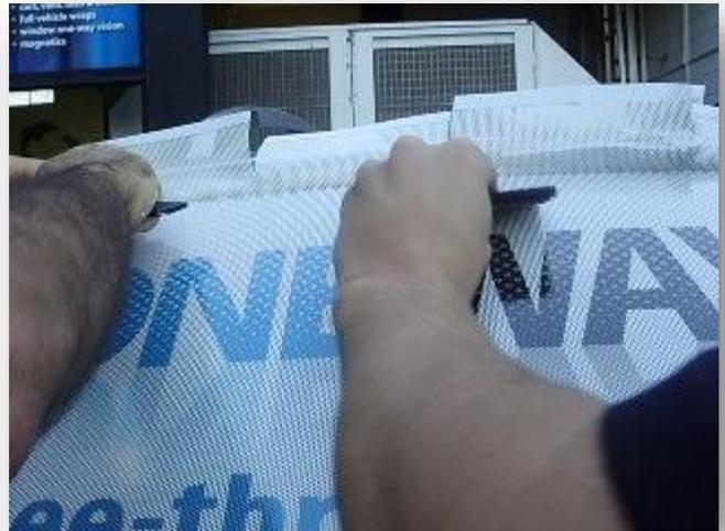
6. Peel one half of the backing release liner from the OWV film. One person will need to hold the OWV face stock up and off the release liner, while the other person cuts the release liner up to the half way (centre) point. Using a cotton glove, wipe away any flecks off the windscreen left after cutting the release liner.
